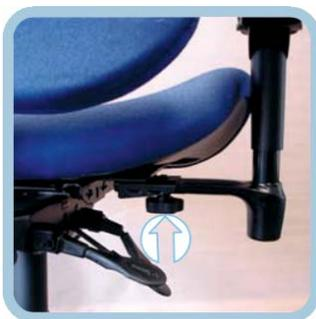
Twist the knob at the base of the arm to loosen the arm width lock. Slide the whole arm in or out. Twist the knob back again to lock the arm. Repeat for the other arm.
