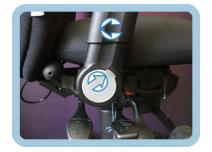
To fold away the armrest, press the button at the bottom of the armrest and fold away the armrest to the rear until it locks into position. To return the armrest to its original position, press the same button and rotate the arm until the button locks back into its upright position.
