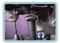
Lift the forward-most lever on the right-hand side to activate the free float. Lower the lever to lock the seat in to position.
