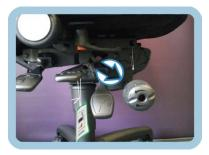
To adjust the body weight tension, twist the knob on the right hand side. Rotate clockwise to increase the tension, rotate anti-clockwise to reduce the tension.
