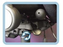
Lift the lever on the rear left-hand side and slide the seat forward or backward. Release the lever to lock the seat depth.
