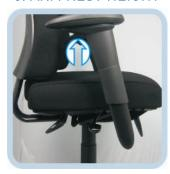
Push in and hold the button on the underside of the arm to release the arm height lock. Raise or lower the arm. Release the button to lock the arm height. Repeat for the other arm.
